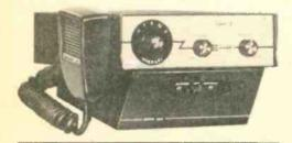
The Portable Station. The Safari II is essentially a miniature solid-state transceiver that can readily be used as a full-power portable because of the many optional accessories specifically intended for portable service.
