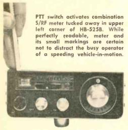
jection. The receiver's sensitivity for a 10 db S+N/N ratio checked out at 0.45 uv. Adjacent channel rejection was 43 db; AGC action for the 74 db input signal variation test was 13 db—not outstandingly good but adequate.
