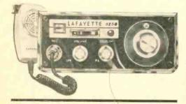
The Mobile Station. The very small size of the Lafayette HB-525B (2½ x 6½ x 8¼ in.) makes it particularly attractive for mobile operation (it's easy to install and remove, and it takes up virtually no leg room).
